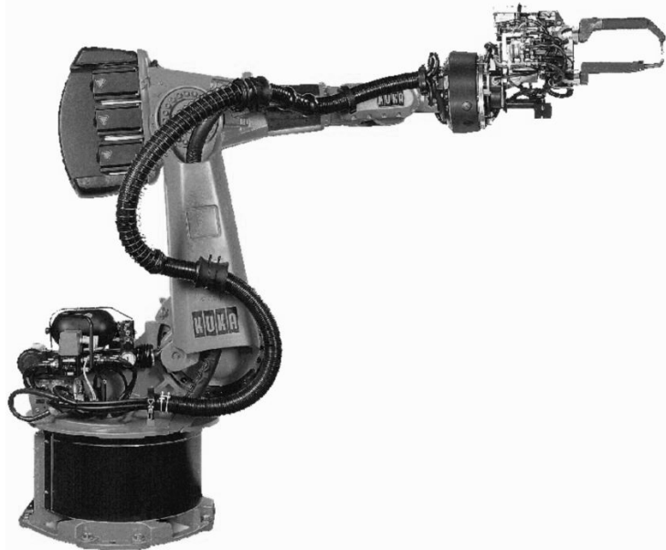
Fig. 2. KUKA KR150 industrial robot with spot-welding tool.
