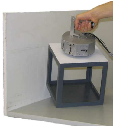
Fig. 10. In the experiment to validate the presented approach a cube is manipulated in contact with three perpendicular faces.
