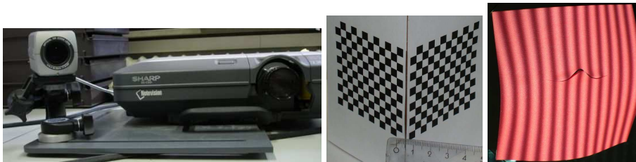
Fig. 4. Setup with camera, projector, calibration box and mockup
